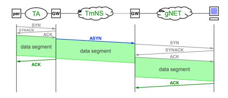
Figure 5: Unreliable connection transfer mode
