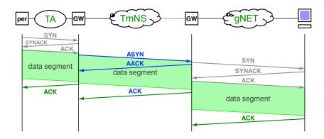
Figure 3: Near-reliable transfer mode
