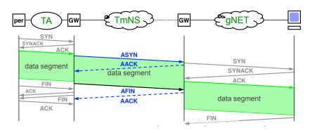
Figure 1: AeroTP connection setup
