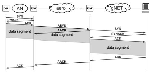
Fig. 8. AeroTP reliable connection transfer mode.
