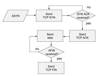
Fig. 6. AeroTP to TCP egress GW conversion procedure.
