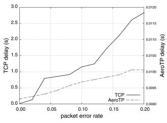
Fig. 14. TCP and AeroTP connection establishment delay.
