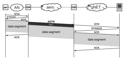
Fig. 10. AeroTP quasi-reliable transfer mode.
