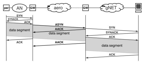
Fig. 9. AeroTP near-reliable transfer mode.
