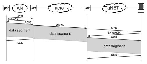
Fig. 11. AeroTP unreliable connection transfer mode.
