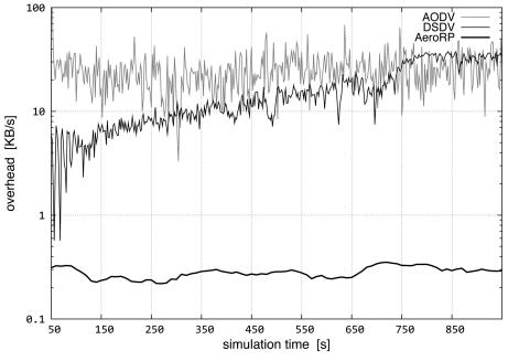
Fig. 19. Routing overhead for Mach 0.3 to 3.5.
