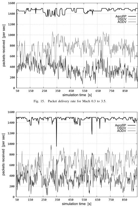
Fig. 16. Packet delivery rate for Mach 3.5.
