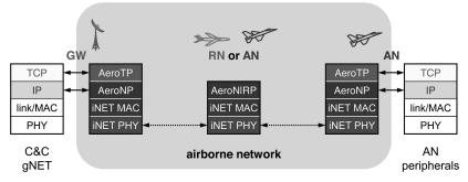
Fig. 2. Airborne network protocol architecture.
