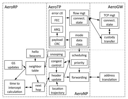
Fig. 3. Airborne network protocol functional block diagram.
