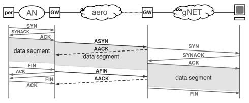
Fig. 4. AeroTP connection setup.
