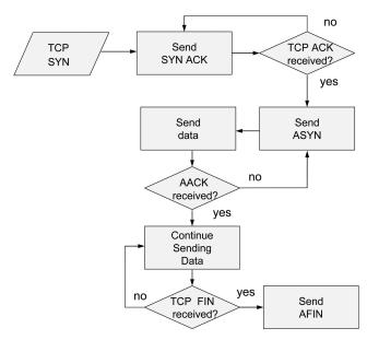
Fig. 5. TCP to AeroTP ingress GW conversion procedure.
